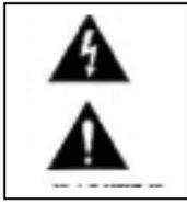
Intended to alert the user to the presence of un-insulated “ dangerous voltage” within the product’s enclosure that may be of sufficient magnitude to constitute a risk of electric shock to persons.
